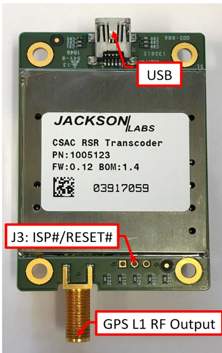
Figure 5.1 Location of ISP and Reset header J3
