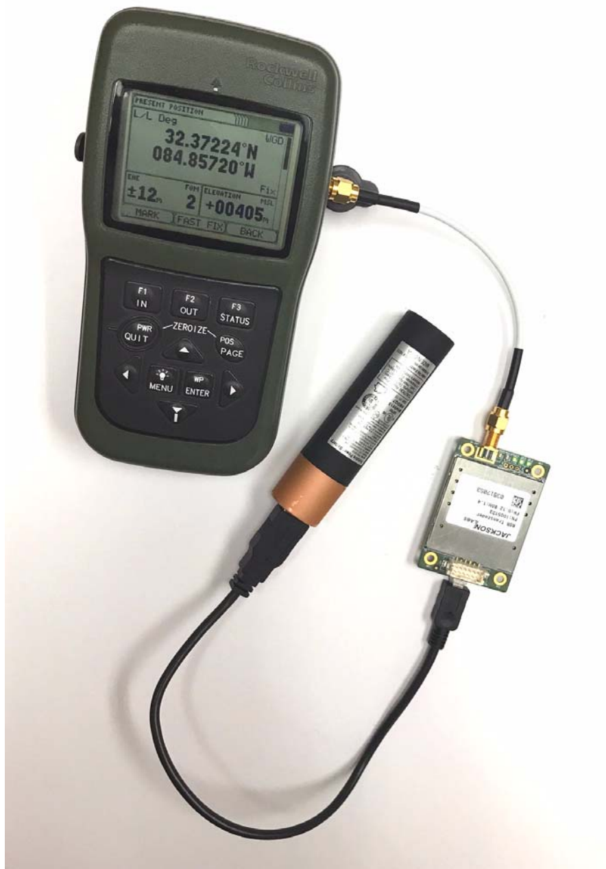
Figure 2.2 DAGR Target Receiver with battery-powered RSR GNSS Transcoder™
