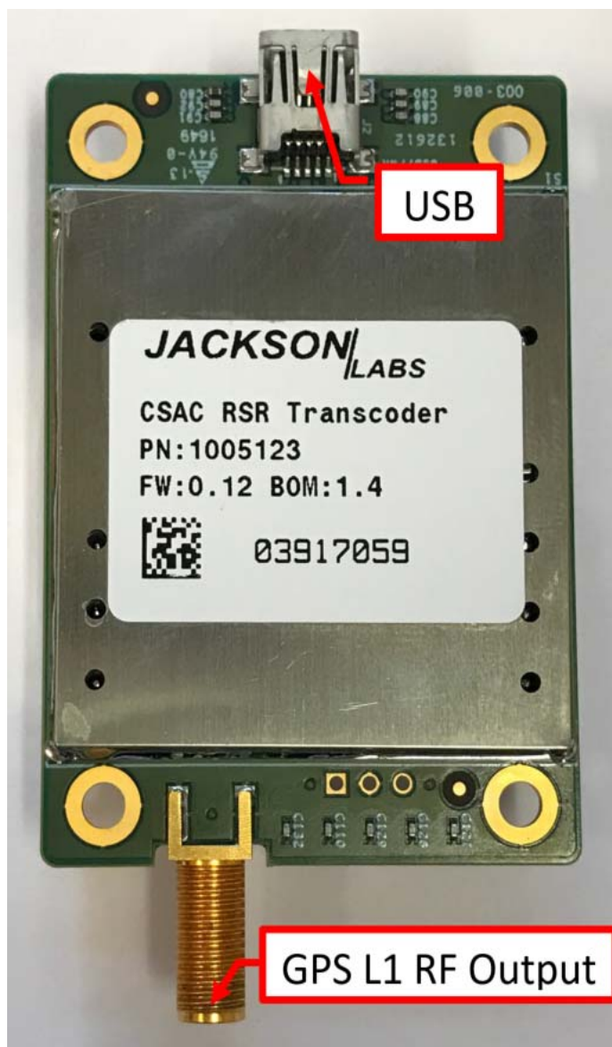
Figure 2.1 Minimum connections to the RSR GNSS Transcoder™ PCB
