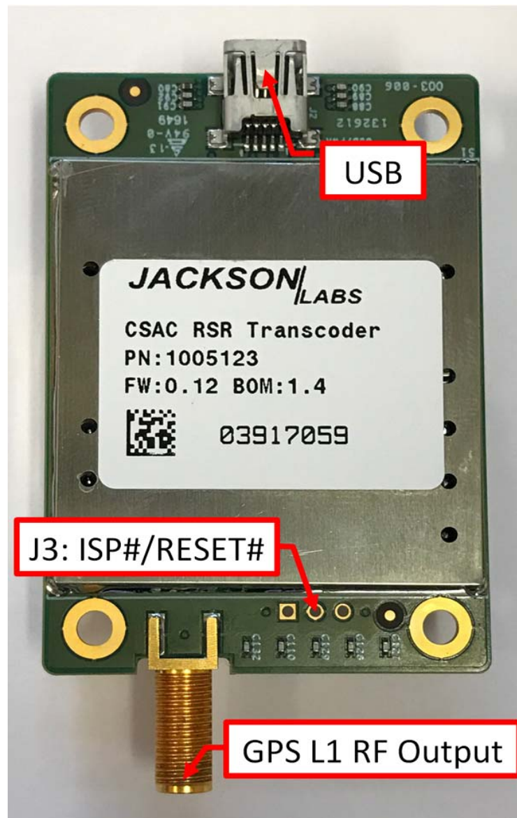
Figure 3.3 Major connections of the RSR GNSS Transcoder™ PCB Bottom Side
